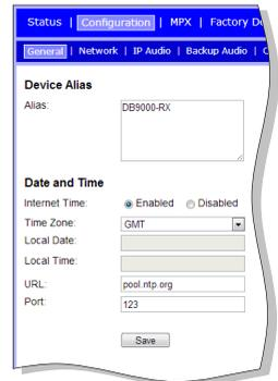
**NOTE:** After selecting new settings, press the SAVE button to put them into effect. Some of the new settings can reset DB9000-RX.
